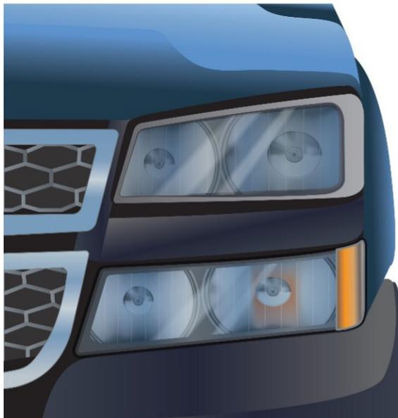
**Figure 1.** GMT 800 “Classic” truck two-piece headlight. Split design is a unique identifying feature
